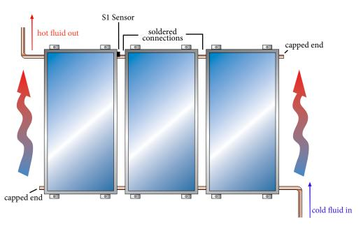
Three solar collectors are connected to each other so that they form one large solar collector array. The collectors have "internal headers" which go across the top and bottom and have outlets on the sides. When the collectors are connected, the headers of each solar collector are soldered to the headers of the others.
