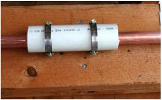
Do not forget the sensor wires. Attach sensor wires to the outside of the insulation to eliminate thermal degradation (*See diagram in controller section*).
