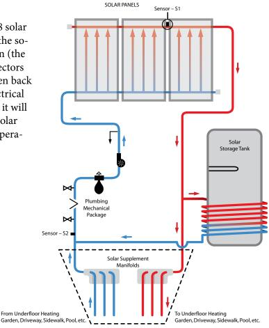
If S1 is greater than S2, the pump comes on and fluid circulation begins between the solar collectors and the tank heat exchanger. When the temperature difference is small, the variable speed pump runs slowly; when the temperature difference is greater the pump runs faster. The variable control feature has many benefits including improved low sun performance, less control cycling and conservation of electrical energy at the pump.
