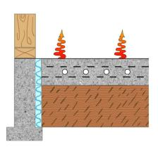
But the choice of insulation method can make a big difference in the ability of the building to store heating or cooling energy. If the insulation is placed vertically, the heat storage ability of the earth is incorporated into the building down to an effective depth of about 3 feet.
