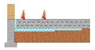
Insulation of decreasing thickness is placed from the perimeter of the slab in towards the middle of the building. It is common to use 2" thick extruded polystyrene for 4 ft and then 1" thick for another 4 ft and then no insulation at all under the center of the slab.
