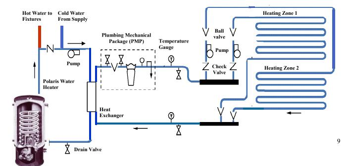
**OPERATION:** When heat is called for by a thermostat, the heater pump comes on and water flows from the water heater through 1 side of the heat exchanger, heating it up in the process. At the same time, the zone pump comes on and causes water (or anti-freeze) to flow through the other side of the heat exchanger to pick up the heat and then travels through the heating zone. When the thermostat in the zone is satisfied, it shuts the pumps off.
