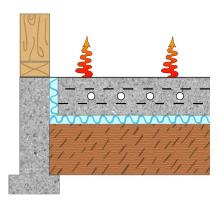
This results in a building that can store large quantities of heating or cooling energy. Such a building can "coast" through the Spring and Fall seasons without large amounts of heating or cooling energy inputs. Such a building can also be designed to store alternative energies such as solar in an efficient and cost effective way.
