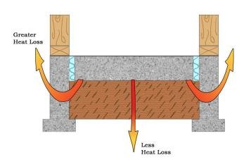
The proper material for below grade insulation is extruded polystyrene. Other materials are prone to absorb moisture or do not have enough compressive strength or stability over time. Some promote a very thin sheet of air-bubbles with foil. This **is not** an acceptable substitute for extruded polystyrene. There is no substitute at present in our opinion.
