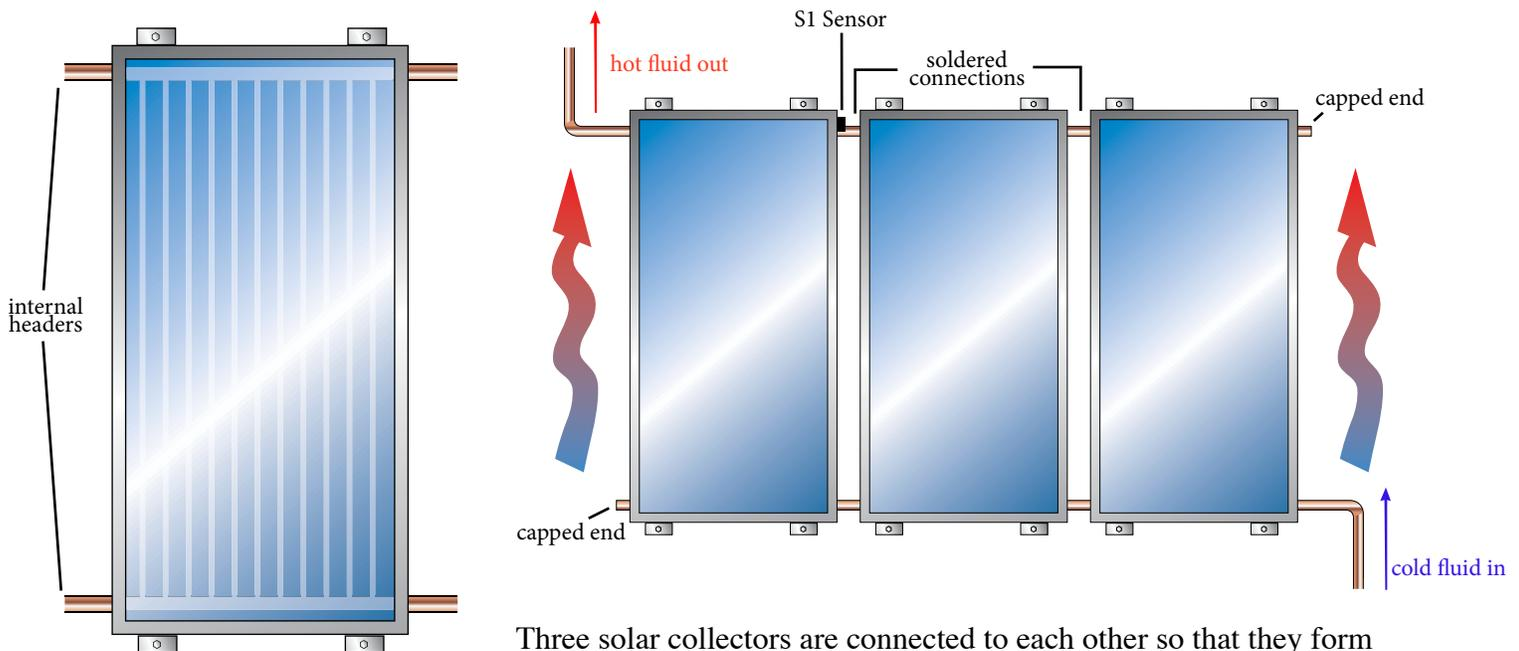
Three solar collectors are connected to each other so that they form one large solar collector array. The collectors have “internal headers” which go across the top and bottom and have outlets on the sides. When the collectors are connected, the headers of each solar collector are soldered to the headers of the others.
