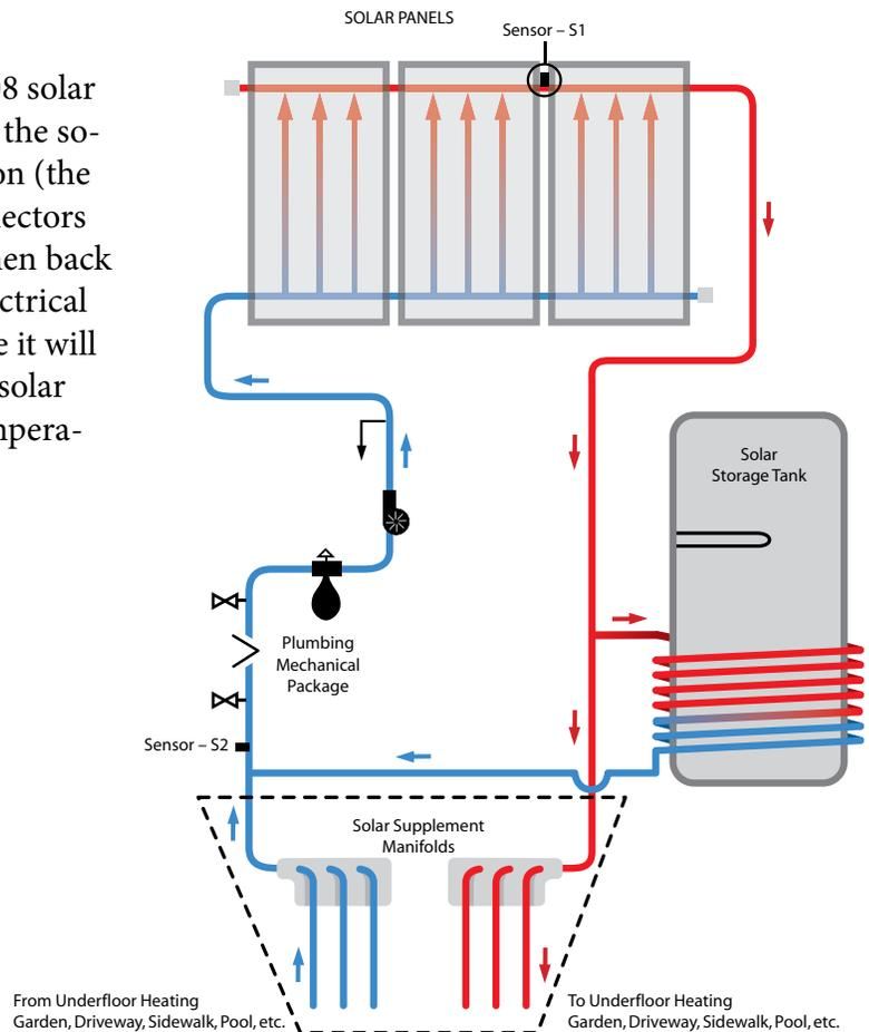
If S1 is greater than S2, the pump comes on and fluid circulation begins between the solar collectors and the tank heat exchanger. When the temperature difference is small, the variable speed pump runs slowly; when the temperature difference is greater the pump runs faster. The variable control feature has many benefits including improved low sun performance, less control cycling and conservation of electrical energy at the pump.
