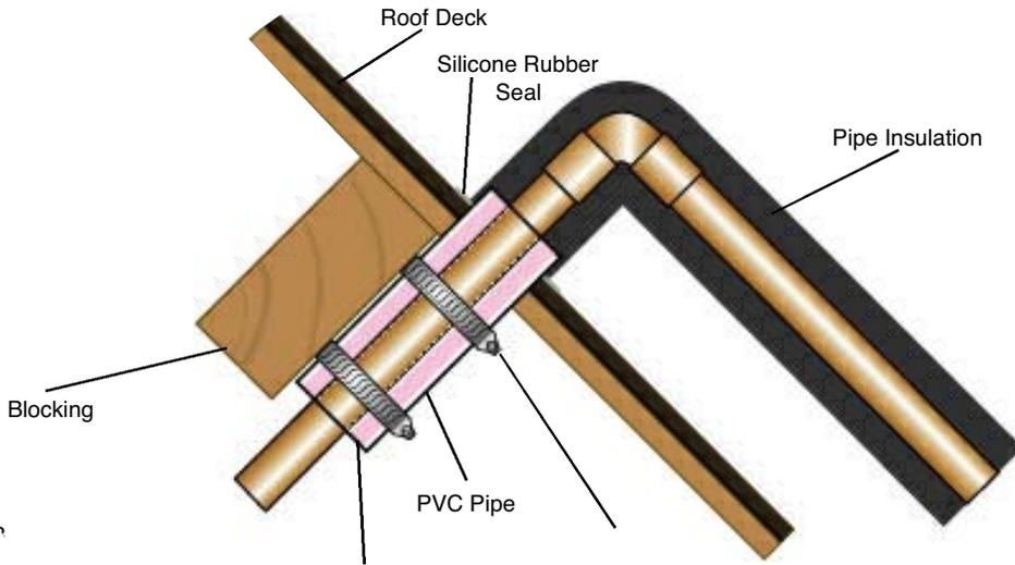
◀ The roof can be penetrated with this detail or with a boot. Seal with silicone sealant, top and bottom and sides.
