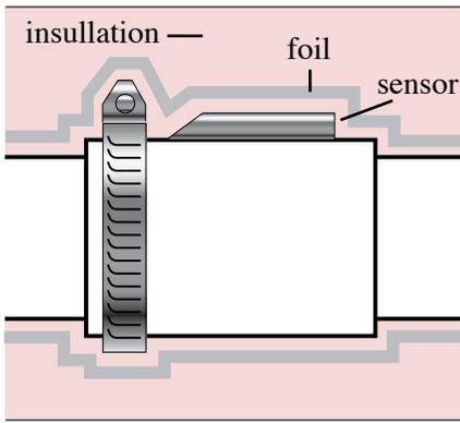
◀ The placement and insulation of the temperature sensors is a very important. Performance can suffer by 20% or more if the sensors are not installed properly.
