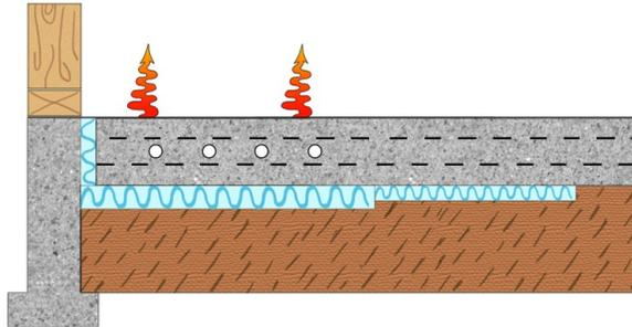
Insulation of decreasing thickness is placed from the perimeter of the slab in towards the middle of the building. It is common to use 2” thick extruded polystyrene for 4 ft and then 1” thick for another 4 ft and then no insulation at all under the center of the slab.
