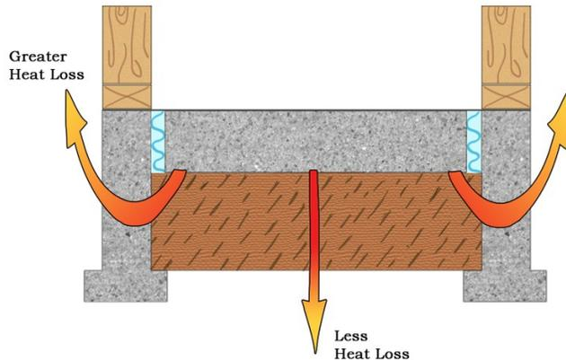
The proper material for below grade insulation is extruded polystyrene. Other materials are prone to absorb moisture or do not have enough compressive strength or stability over time. Some promote a very thin sheet of air-bubbles with foil. This **is not** an acceptable substitute for extruded polystyrene. There is no substitute at present in our opinion.
