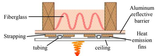
**LEDGER** – Tubing is placed upon a ledge within the joist space. This is a common retrofit solution when building up the floor is not practical. **R**
