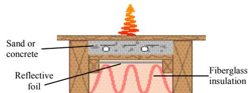
**BETWEEN STRAPPING** – Tubing is placed in the space between wooden strapping members. If the space is filled with concrete or dry mix, the method offers most of the performance of slabs, and yet allows wooden flooring to be placed on top. A good way to heat a “great room” with high heat requirements.
