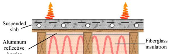
**TOPPING SLABS** – A slab containing heating tubes is cast over an existing slab. **R**
