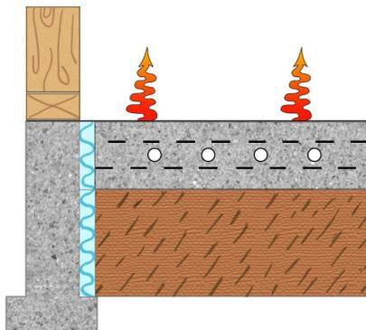
But the choice of insulation method can make a big difference in the ability of the building to store heating or cooling energy. If the insulation is placed vertically, the heat storage ability of the earth is incorporated into the building down to an effective depth of about 3 feet.
