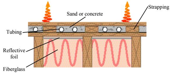
**ON TOP OF THE SUBFLOOR** – Ply-wood is ripped into strips and placed on top of the floor leaving a groove wide enough for an aluminum heat emission fin and the tubing. **R**
