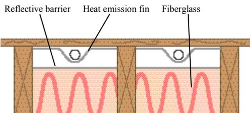
This detail ensures that most of the heat given off by the floor will go up. An aluminum reflective barrier reflects radiant heat that is headed downward back up to the floor. The effectiveness of the aluminum foil can be lowered by dust accumulation. Plastic sheeting or rosin paper can be applied under the finish floor to eliminate dusting.
