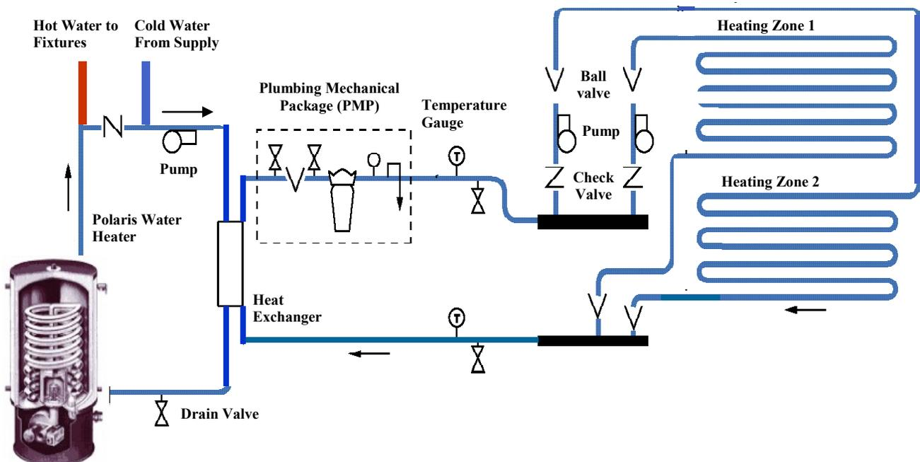
**OPERATION:** When heat is called for by a thermostat, the heater pump comes on and water flows from the water heater through 1 side of the heat exchanger, heating it up in the process. At the same time, the zone pump comes on and causes water (or anti-freeze) to flow through the other side of the heat exchanger to pick up the heat and then travels through the heating zone. When the thermostat in the zone is satisfied, it shuts the pumps off.
