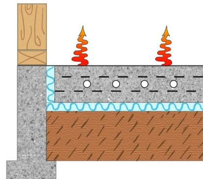
This results in a building that can store large quantities of heating or cooling energy. Such a building can “coast” through the Spring and Fall seasons without large amounts of heating or cooling energy inputs. Such a building can also be designed to store alternative energies such as solar in an efficient and cost effective way.
