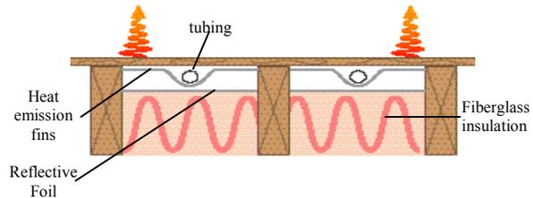
**CEILING** – Tubing is placed between strapping underneath the ceilings.
