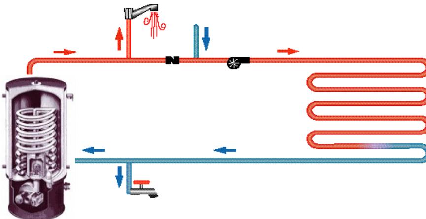
*The Radiantec Open Direct System provides space heating and domestic hot water from a single heating appliance.*
